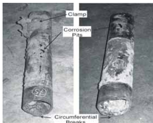
Figure 14. Multiple failures on same pipe. (City of Toronto)
