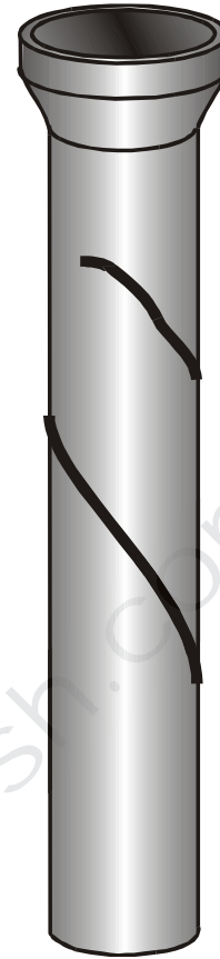
Figure 3. Spiral failure mode in mid-diameter (380 mm –500 mm) pipe. Corrosion pitting failures have also been seen in these pipes.
