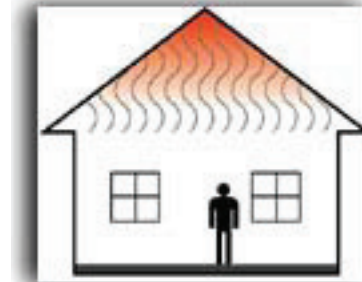
Heat profile with Traditional Convection Heating
