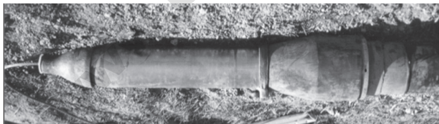
Figure 2 The Bursting Head of the Pneumatic System
