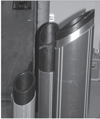
Figure 22 Protecting the PE Pipe from Shards
